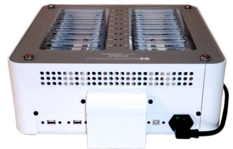
Rear view: dock can be adjusted for anything from a naked iPod™ to an iPhone™ 8+ in an OtterBox™
