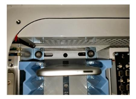
The device should center in the V groove when properly positioned
