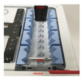
Loosen the front and back screws (1/4 to ½ turn) on one guide assembly. It should snap inward. Loosen the screws for the second guide assembly in the same manner. The guides are "sprung" to help center and position the guides in relation to the connectors on the base. Use the Allen key to tighten the two front and two rear socket screws.
