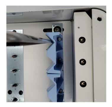
The device should center in the V groove when properly positioned
