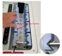
The device should center in the V groove when properly positioned.
